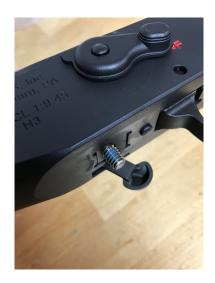
Place the aluminum housing against the bottom of the receiver so that the front "ears" surround the magazine catch assembly and apply pressure towards the muzzle to ensure that it the housing is seated against the magazine catch assembly. With the aluminum housing in place, thread in and tighten the 1/4-20 cap screw with the 3/16 hex key. At this point, the KNS delete kit is installed and all that is left is to install an AR15 pattern grip and reassemble the weapon.
