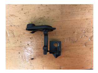
Apply a small amount of medium thread locker to the \*STAINLESS\* 1/4-20 cap screw provided in the kit and place it into the bell crank nut from the top, down so that it protrudes from the bottom of the receiver. Engage this screw with a 3/16 hex key to hold both the screw and bell crank nut in place.
