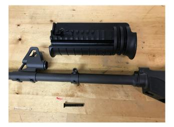
Use a large common type screw driver to remove the front magwell screw, taking care to keep tool fully engaged under load as this fastener usually thread-locker applied.
