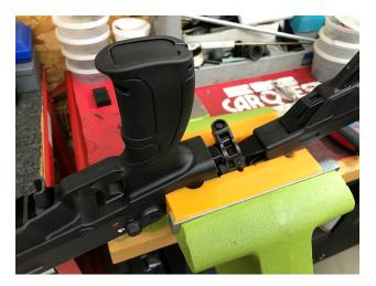
Using the tip of your screwdriver - open the compartment on the bottom of the pistol grip.
