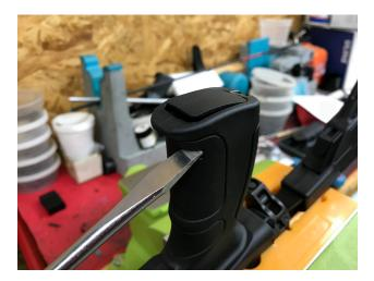
Using a common type screwdriver with an extra wide tip, engage the grip screw - use an adjustable wrench to apply torque to the screwdriver, while applying downward pressure to keep the screwdriver tip fully engaged. This screw is usually very tight and it is important to keep the screwdriver fully engaged while torque is being applied, otherwise damage to the screw can occur. Remove the grip screw and set aside.
