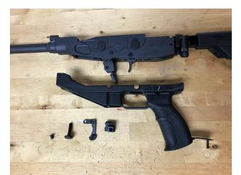
Re-insert left safety lever into the receiver from the bottom, then partially re-install right side safety selector. The lower boss on the safety sector lever must be engaged with the hole in the end of the left safety lever. Getting these to parts to engage each other, while at the same time reinstalling the right selector lever is a challenge if you've never done it before, so do not be frustrated if it takes a few tries.
