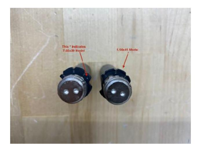
At this point, typical installation is complete, all that is left is to test fire the weapon in all configurations to determine best setting(s).| One of the many great features of the CZ Bren2/806<sup>TM</sup> platform is the three user-selectable gas apertures between the barrel and the piston journal. These allow the hard aperture size to be changed by the user to accommodate different configurations/ammunition types simply by turning the CzechValve body within the gas block.
