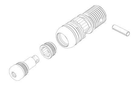
Exploded view of the piston assembly and bolt carrier nose, showing the adjustment collar and two 'jet insert' options
