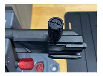
Once the thread locking compound has set, the installation is complete. There are currently two options for handles, one with a strait fluting and one with a "waffle" texture. Both handles install and function the same way, the "waffle" style is shown here.
