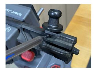
The factory uses a potting compound resembling thread locking compound. In order to successfully remove the factory charging handle - this compound must be heated to the point of failure, and the handle gently lifted out of the carrier.
