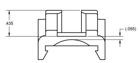
Using a .250 end mill, cut a slot to these specifications to allow a KNS AK Precision Rear Sight to be installed in a Sabrewerks KOP iron sight adapter base.
