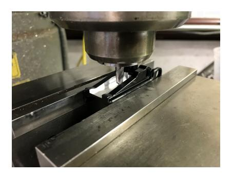
In this photo, you can see a typical fixturing layout for this operation, the preferred cutting tool is a .250" diameter end mill suitable for aluminum.
