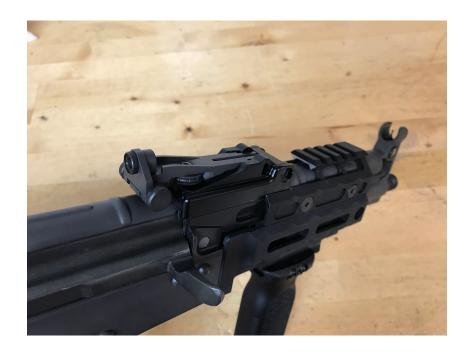
The KOP iron sight adapter assembly may now be installed onto the KOP rear sight base per Sabrewerks' installation instructions.
