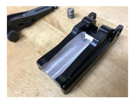
In this photo, a clearance cut can be seen where there is shiny/bare aluminum. This cut replicates the casting void present in a standard AK rear sight tower and allows the KNS sight to correctly nest in the mount.
