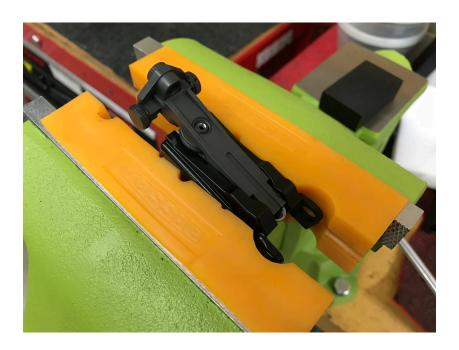
Once the milling operation has been completed to print, the KNS sight may be installed in the same manner as any factory AK rear sight by compressing the spring and sliding the sight into the base.
