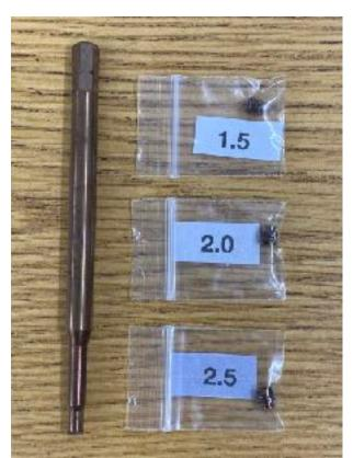
If more energy is desired, install the gas jet with the next size larger port, if less energy is desired, install a smaller than factory jet. Think of this like the transfer case on a manual transmission - you are modulating the total volume of gas available for the regulator to...regulate.
