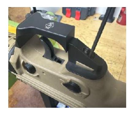
Once the plastic delete has been secured to the host firearm, the pistol grip can be installed. The KNS X-95 plastic delete provides an AR15-compatible interface - however, the X-95 has geometry that exceeds the internal width of the slot in a standard AR15 compatible grip.
