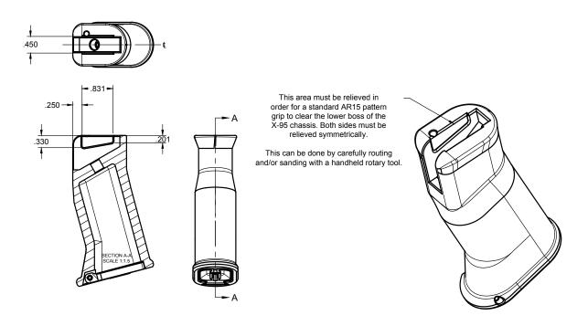
Grips with a "spur" must also be modified to remove the "spur".
