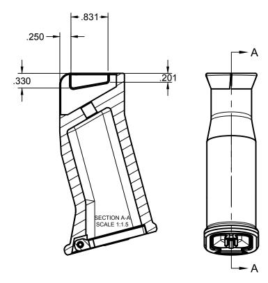
This area must be relieved in order for a standard AR15 pattern grip to clear the lower boss of the X-95 chassis. Both sides must be relieved symmetrically.
